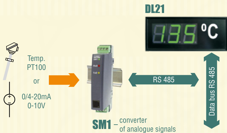
Measurement and visualization of temperature from Pt100 sensor or from standard analogue signals
